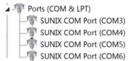
DevicePort® supports physical COM port mapping over Ethernet connection
