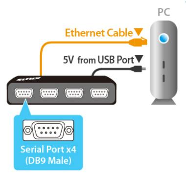
With Ethernet hot-plug and system auto-detect capability, user can expand RS-232 COM and Printer LPT port easily without complex software configuration. Just plug RJ45 Ethernet cable between SUNIX DevicePort® and PC host side, system will create physical COM/LPT ports automatically with real time data transmit and receive communication. User can easily access port by using existing software and application, no longer TCP sock protocol compiling.
